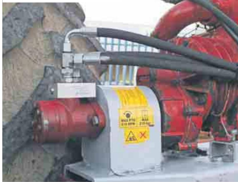
to start slowly and to prevent shock loading in the system, an anti-cavitation block is fitted which alters the oil flow on start-up and stopping, making it smoother.
