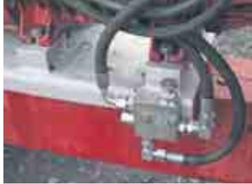
An optional manual or electronic flow controller can be specified to alter the oil flow and speed at which the pump runs when using different tractors.
