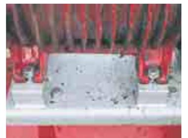
The kit bolts down to the pump's original bolt holes. The pump is then bolted to the plate, eliminating any need for welding.
